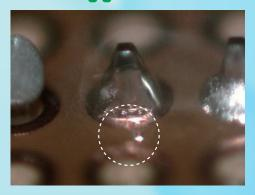
Voids are suppressed by efficiently discharging outgas and eliminating bubbles in the solder.
